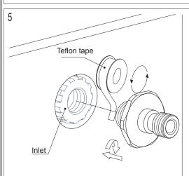
Wrap connector with teflon tape,screw to inlet and close to the finished metope.
